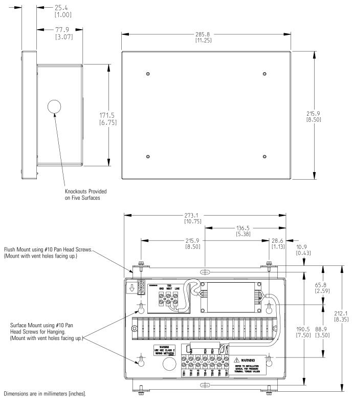
Figure 5-14. Supervisory Contact Module II Dimensions
